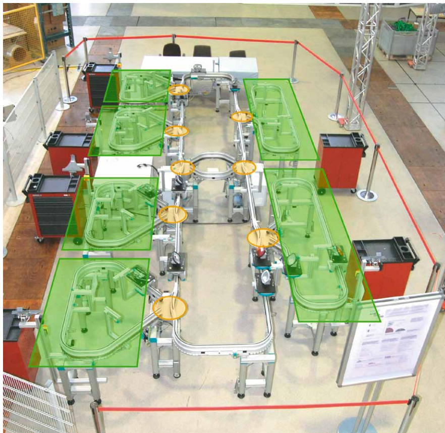
Figure 1: An agent-based assembly system for several variants of an automotive tail-light with five workstations (green) and several rotating switches (yellow). [20]
